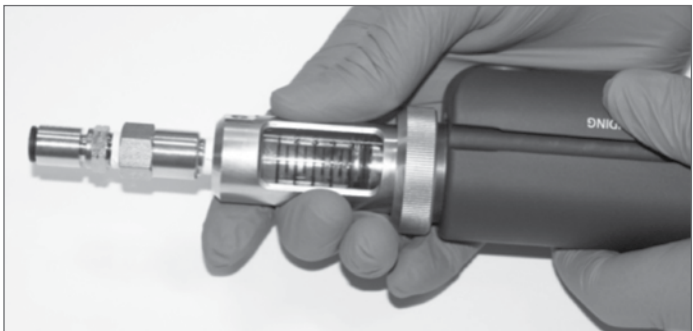
Turn the Glass Barrel until all of the measurement readings are lined up and centered.
