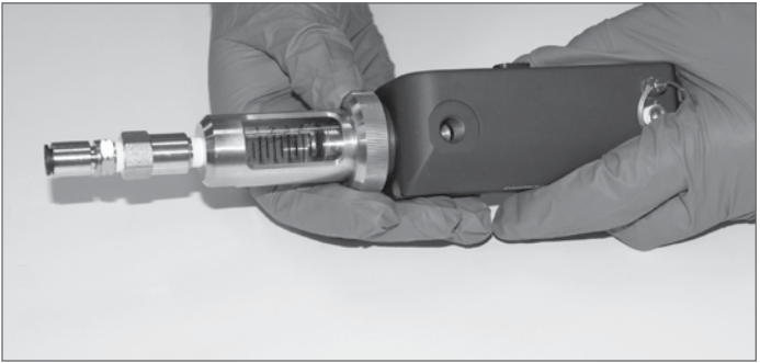
Put the Case ring back over Glass Barrel Case and turn clockwise. Do not tighten yet.
