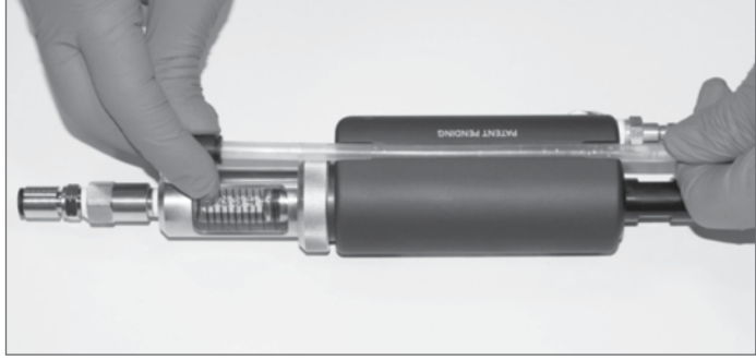
Slide tubing through main body and push it in the Push-to-Connect (PTC) fitting.
