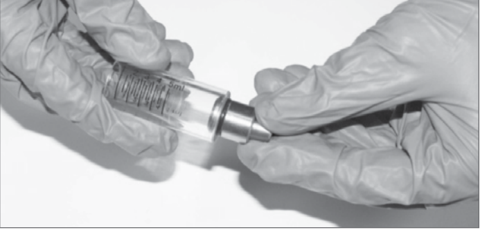
Push the Glass Barrel back onto the Piston. Ensure that grease is applied to Piston after each use.
