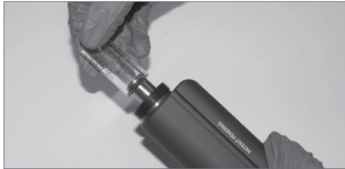
Pull Glass Barrel away from Piston.
