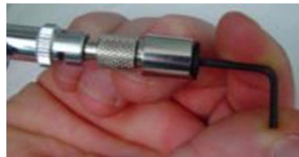
PTC fittings use a 5/16" hex tool for installation and removal.
