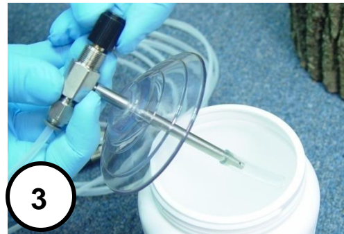
3. Attach the Tip Guard. Turn each STINGER ON, and OFF to Prime Supply Lines.
