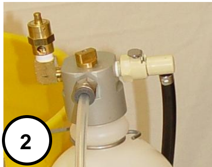
2. Pressurize Tree I.V. Make sure valves are OFF.
