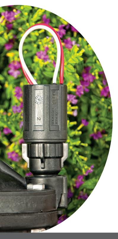
DIG's Unimax S-305DC solenoid is a two-way magnetic latching solenoid with the ability to adapt to various brand name valves using DIG's assortment of threaded adapters. The solenoid can also operate with various two-wire DC controllers available on the market to a distance of up to 200 ft using 14-AWG wire. The S-305 uses a sealed plastic over-molding to prevent water or contaminants from entering the solenoid housing. The normal actuation of the S-305 is via a bidirectional pulse.
