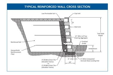
the wall. Place the front edge of the geogrid on the designated course a maximum of one (1) inch from the face of the unit. Apply the next course of units to secure it in place. Pull the reinforcement taut and secure in place. A minimum of six (6) inches of backfill over the grid is required prior to vehicular operation.
