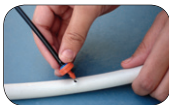
Step 2: Insert the dripper assembly into the tubing.
