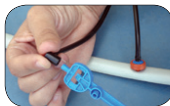
Step 3: Attach spray stake to dripper assembly.
