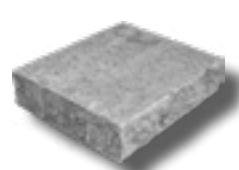
Parapet Cap 3 5/8" x 15 5/8" x 13" wt: 56 lbs. qty/pallet: 45
