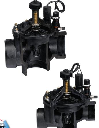
The new P-220S Scrubber Series valves feature Toro's patented Active Cleansing Technology (ACT™) system. The ACT system's durable turbine is in constant rotation, which in turn keeps the metering and filtration area free of dirt and algae build-up. The turbine is constructed of materials resistant to chlorine, chloramines, and ozone, thereby keeping the valve operating at peak performance.
