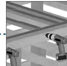
Connect with self-tap- ping screw (ST02)
