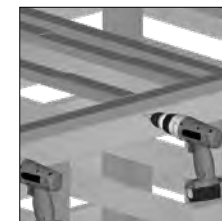
Connect with self-tapping screw (ST02)
