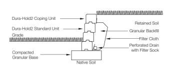
Cross sections are examples, and must not be used for construction.
