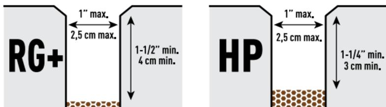
Minimum required depth and maximum width
