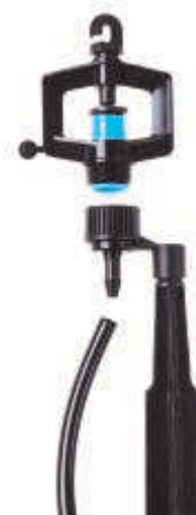
Mini spinner sprinkler (7436) with press fit stake (2010), press fit connector (1032N), and .270" O.D. flexible vinyl distribution tubing
