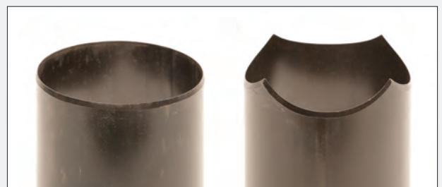
Outside sharpened: push up native soil
