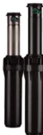
I-25-06 Overall height: 10¼" Pop-up height: 6" Exposed diameter: 1¾" Inlet size: 1"
