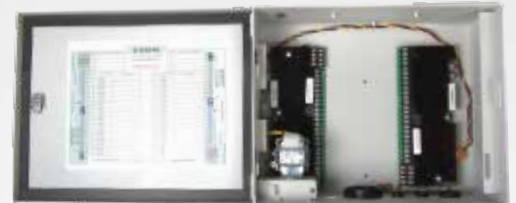
Add additional Powered biCoders installed in separate enclosure
